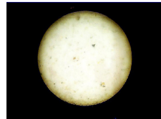
Fluid sample before filtration (NAS 8)
