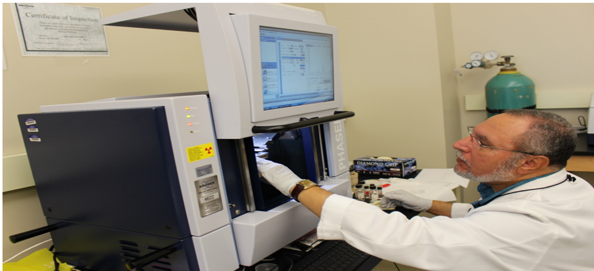
IMAGE 12: PLACING TARBALL SAMPLES IN X-RAY DIFFRACTION MACHINE
