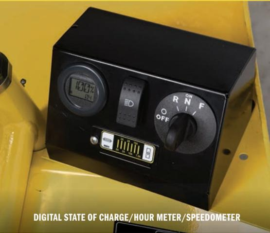
DIGITAL STATE OF CHARGE/HOUR METER/SPEEDOMETER
