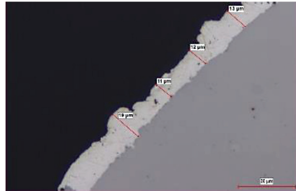
Fig. 1 — Cross section micrograph of the silver coating on stainless steel.
